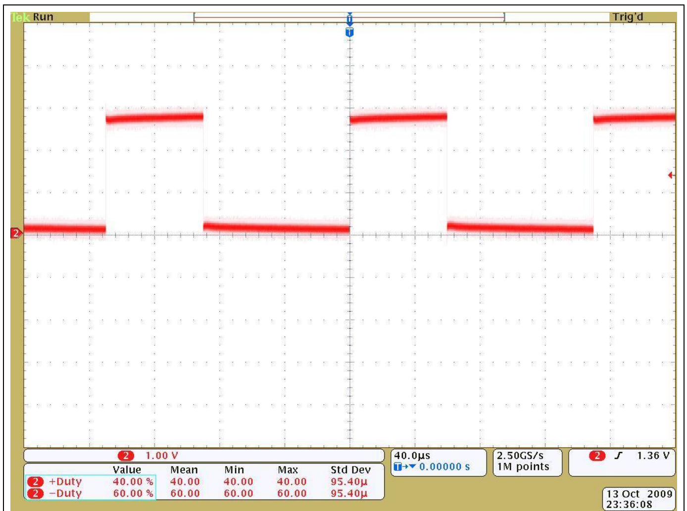
Figure 15. OneNAND checksum failure waveform
